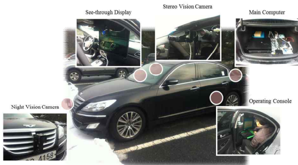
Figure 5. Vehicle AR Information System H/W Installation
